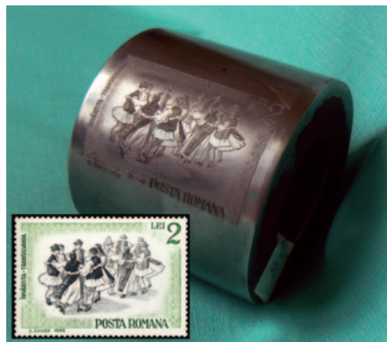
Fig. 7 - Steel cylinder engraving and postage stamp with the face value of 2 lei from the „Folk Dances” 1966, printed in the "taille-douce" (steel engraving) - National Philatelic Museum.
