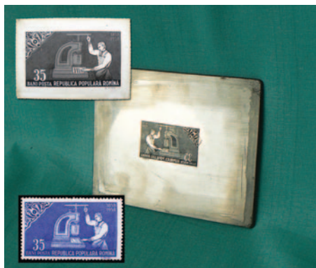
Fig. 6 - Stamp with a face value of 35 Bani from the „Centenary of the Romanian postage stamp” 1958, printed in the "taille-douce" (steel engraving), graphic layout of stamp and engraved steel plate in the negative (National Philatelic Museum ).
